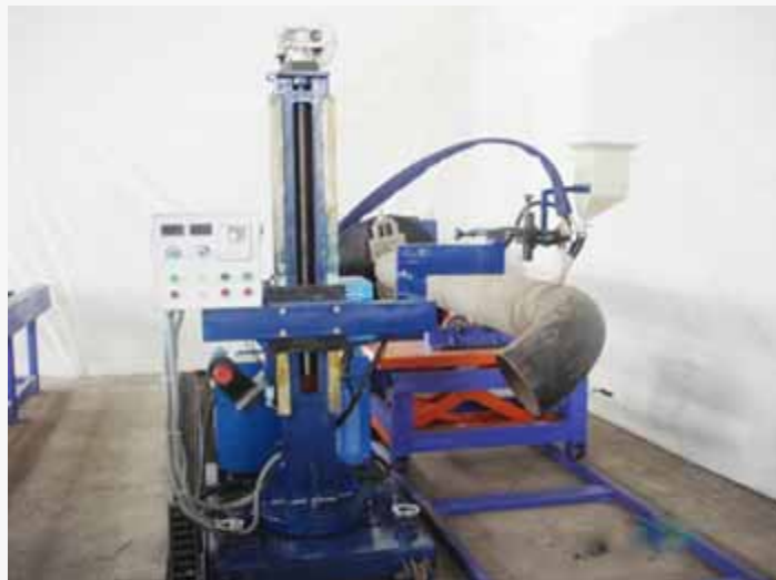
Piping Cantilever Automatic Welding Machine(SAW)
