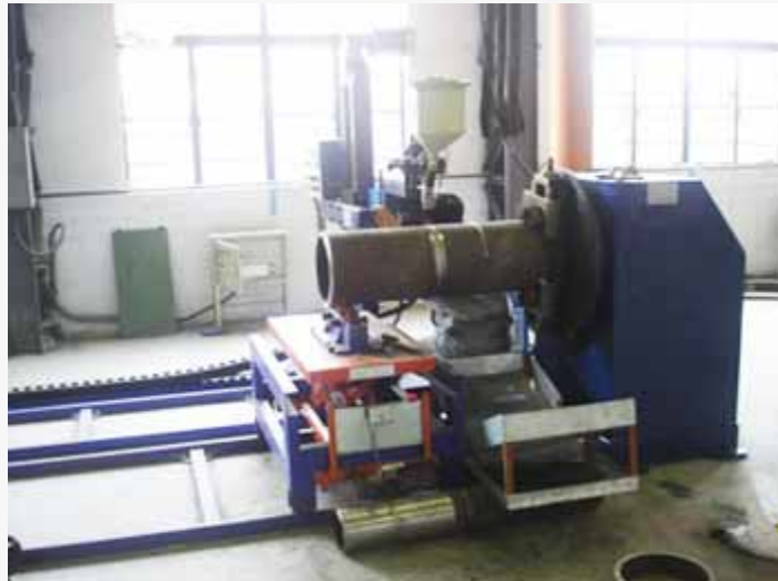
Piping Cantilever Automatic Welding Machine(SAW)
