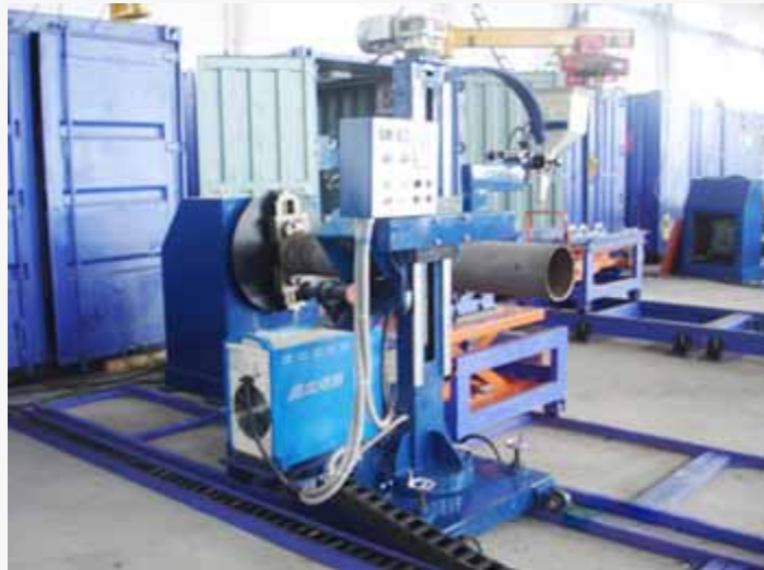
Piping Cantilever Automatic Welding Machine(SAW)
